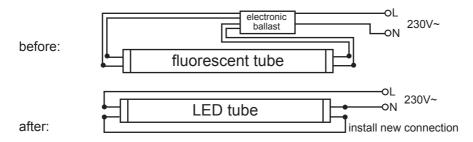
The mounting direction of the LED tube is optional in both cases.
