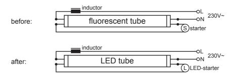
B. Remove the fluorescent tube from the socket and the electronic ballast from the circuitry and connect the LED tube according to the wiring diagram with suitable equipollent and insulated cable pieces. Place the LED tube into the sockets and turn it by 90 degrees.
